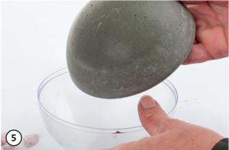
Remove the outer half of the ball. Allow residual moisture to dry completely.
