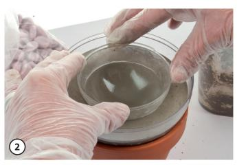
Place the smaller ball half centered on the concrete layer. Pour out the resulting intermediate gap with concrete.
