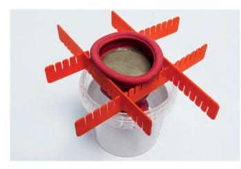
3. Hang the latex mould into a bucket/ box using the mould holder.
