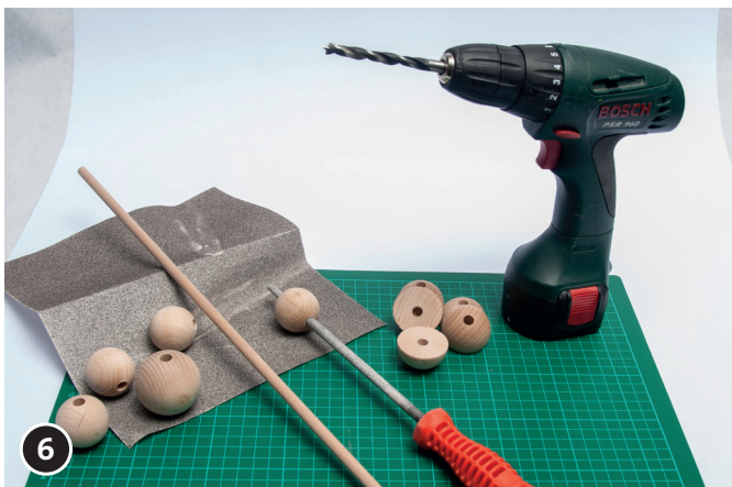
6 With the wood drill bore holes \varnothing 8 mm again into the wooden balls and half ball buttons.
