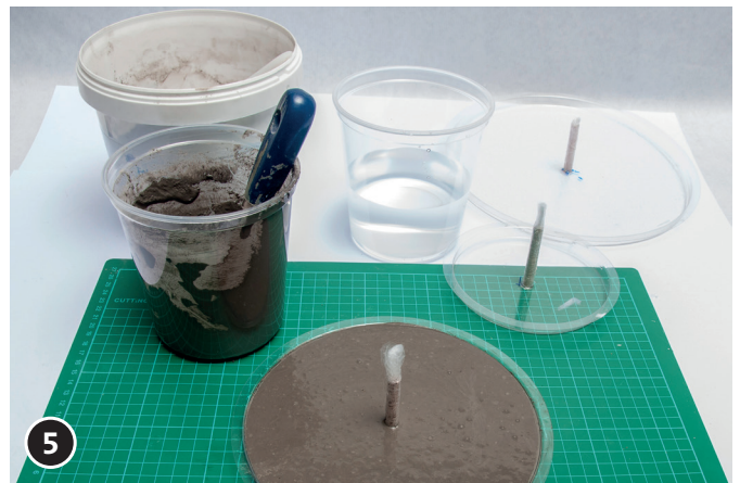
5 Cast concrete according to basic instruction. Remove dowels after drying.
