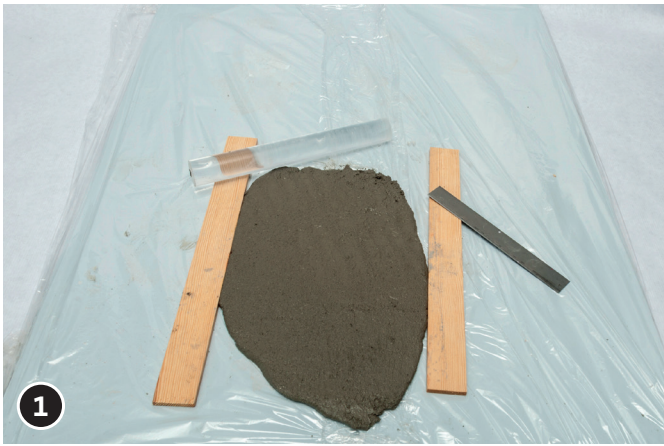
1 Mix kneading concrete according to product instructions. Roll out a 5 mm thick kneading concrete slab.
