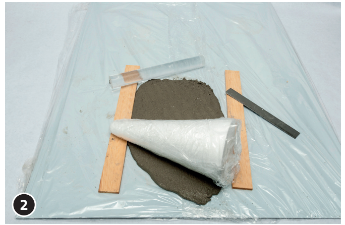
2 Wrap plastic wrap around the polystyrene cone. Place the kneading concrete slab around the cone.
