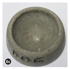
After 24 hours remove the concrete from the bowl. Remove the letters and the half-sphere. Let the remaining dampness dry out properly.
