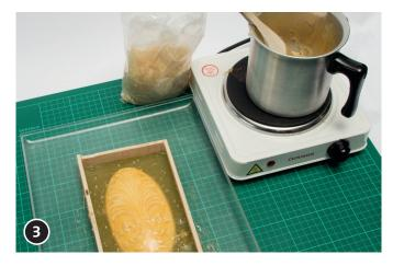
Unfortunately, it is not heat-resistant and resistant to materials containing water. Therefore, the mould can be melted again any time, which offers unique advantages over other similar moulding mixtures. An unsuccessful or imperfect mould can be melted again.
