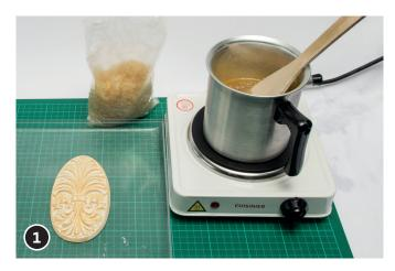
Formaform is a moulding mixture with great application possibilities. Formaform consists of small, rubbery pellets which are heated and melted in a pot with water, just like wax. This produces a thick liquid mixture, which should be mixed with the included Formaform-Liquid at a ratio of 100 : 40.
