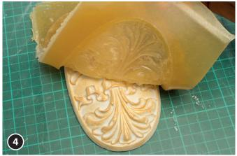
Once the mould is perfect, the included Formaform Thermolan is used to make the mould heat and water-resistant. Brush the inside of the actual mould surface with Formaform Thermolan. Afterwards the mould can be used like any other mould, but can no longer be melted down.
