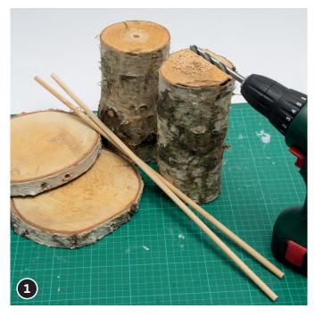
Drill a hole approx. Ø 10mm centrally in the top of the birch trunk. In the lower outer edge of the birch discs as well. Shorten the round wood rods to the desired length.
