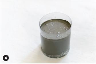
Pour the concrete into a mold. The shape of the doorstop depends only on you.
